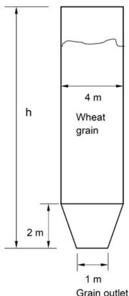
A circular grain silo with conical bottom, as shown in figure, is filled with wheat (true density  $1200 \text{ kg m}^{-3}$ ) with porosity of 0.6. Five hundred metric tonne of wheat fills 80% of its capacity (by volume). The total height ( $h$ ) of the silo from its grain outlet end in m is \_\_\_\_\_.
